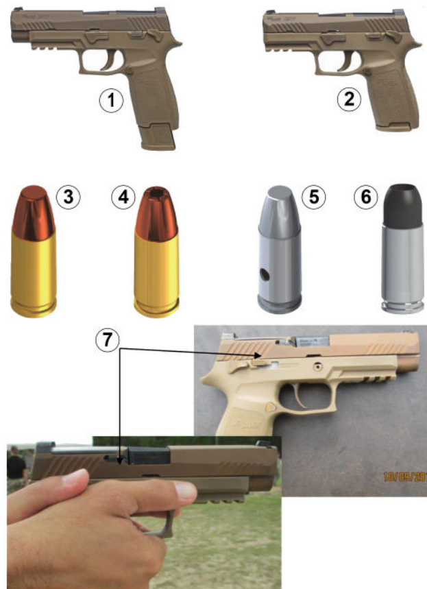
1 - XM17, Full Size, with 21-round magazine 2 - XM18, Compact, with 17-round magazine 3 - XM1152 Ball round 4 - XM1153 Special Purpose (SP) round 5 - XM1156 Dummy round 6 - XM1157 Blank round 7 - Slide Catch Lever
